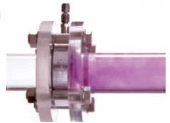
Figure 1. CompaX static mixer with purple additives. Complete mixing at about 3D downstream of static mixer.
